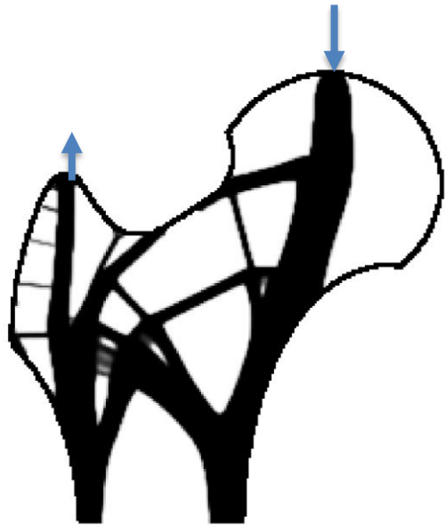
Infill by standard topology optimization
