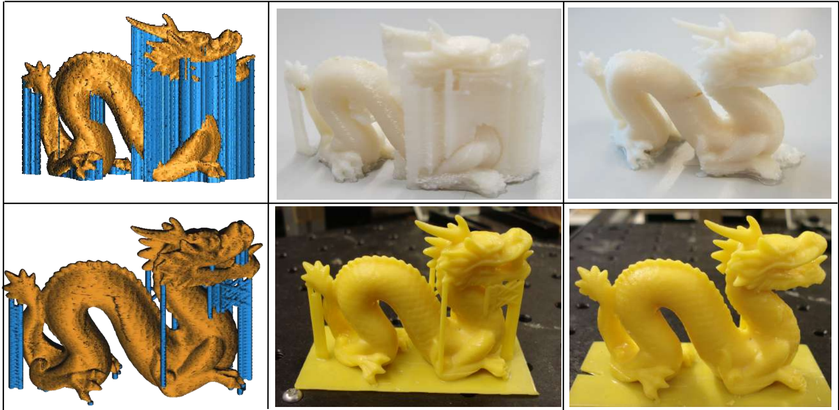
Direct slicing and support generation resultant contour
